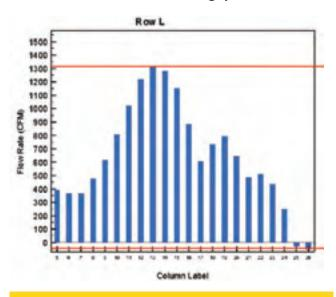
Airflow analysis across one row of racks using floor mount precision air conditioners with 18-inch raised floor.
