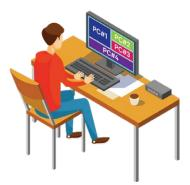
Secure multiviewer KVMs can be used either to access multiple compute resources on a single workstation or project them on a video wall in secure environments, such as command centers.
