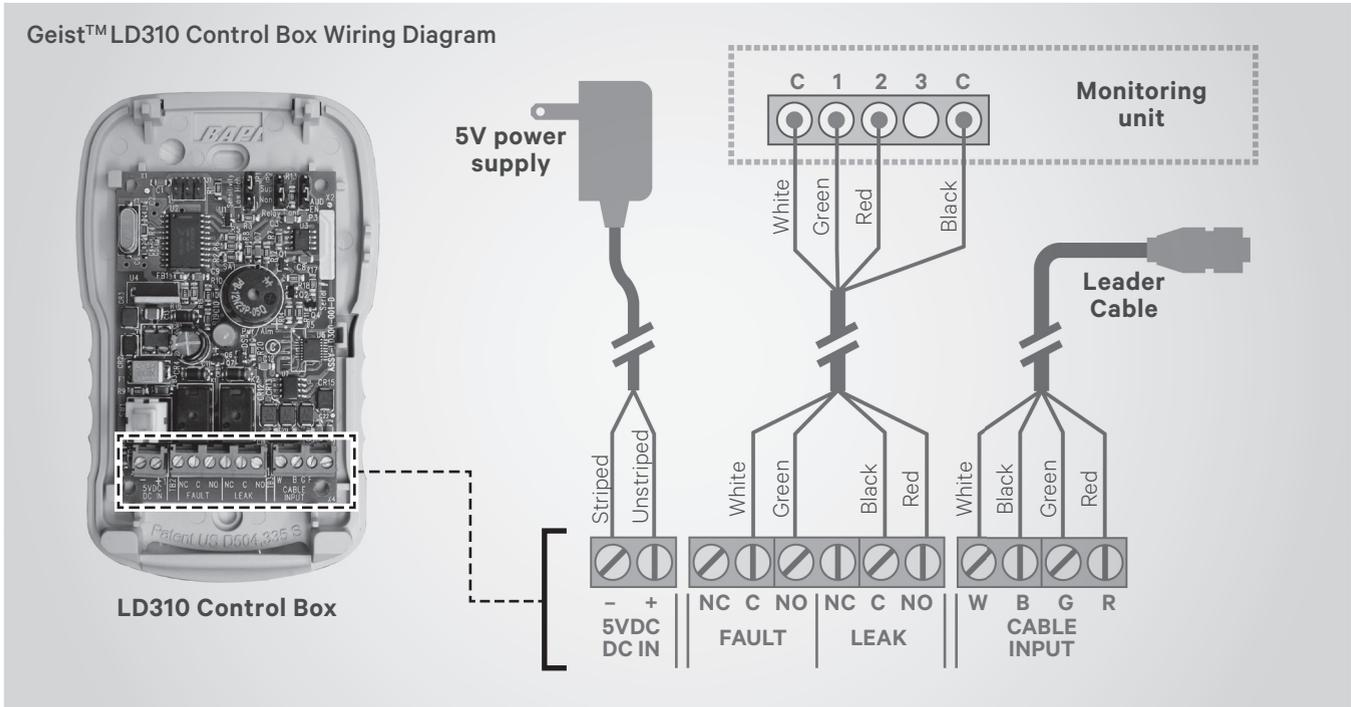
are stripped so that approximately ¼ inch (7 mm) of bare wire is showing. Then insert the wires into the appropriate terminals of the CABLE INPUT terminal block and tighten the screws to lock the wires into place.
