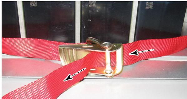
3. Then loop the strap into the outer slot of the buckle. Refer to **Figure 29**.
