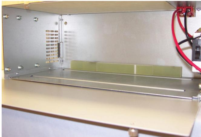
2. Take the (3) Inner Battery Spacers and break off the end portion of the spacer where indicated, as shown in **Figure 21**.
