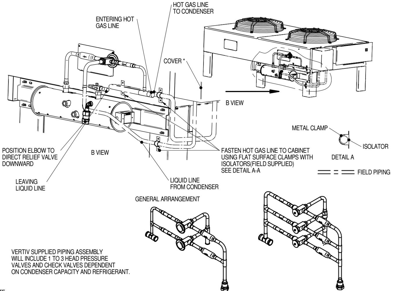
VERTIV SUPPLIED PIPING ASSEMBLY WILL INCLUDE 1 TO 3 HEAD PRESSURE VALVES AND CHECK VALVES DEPENDENT ON CONDENSER CAPACITY AND REFRIGERANT.
