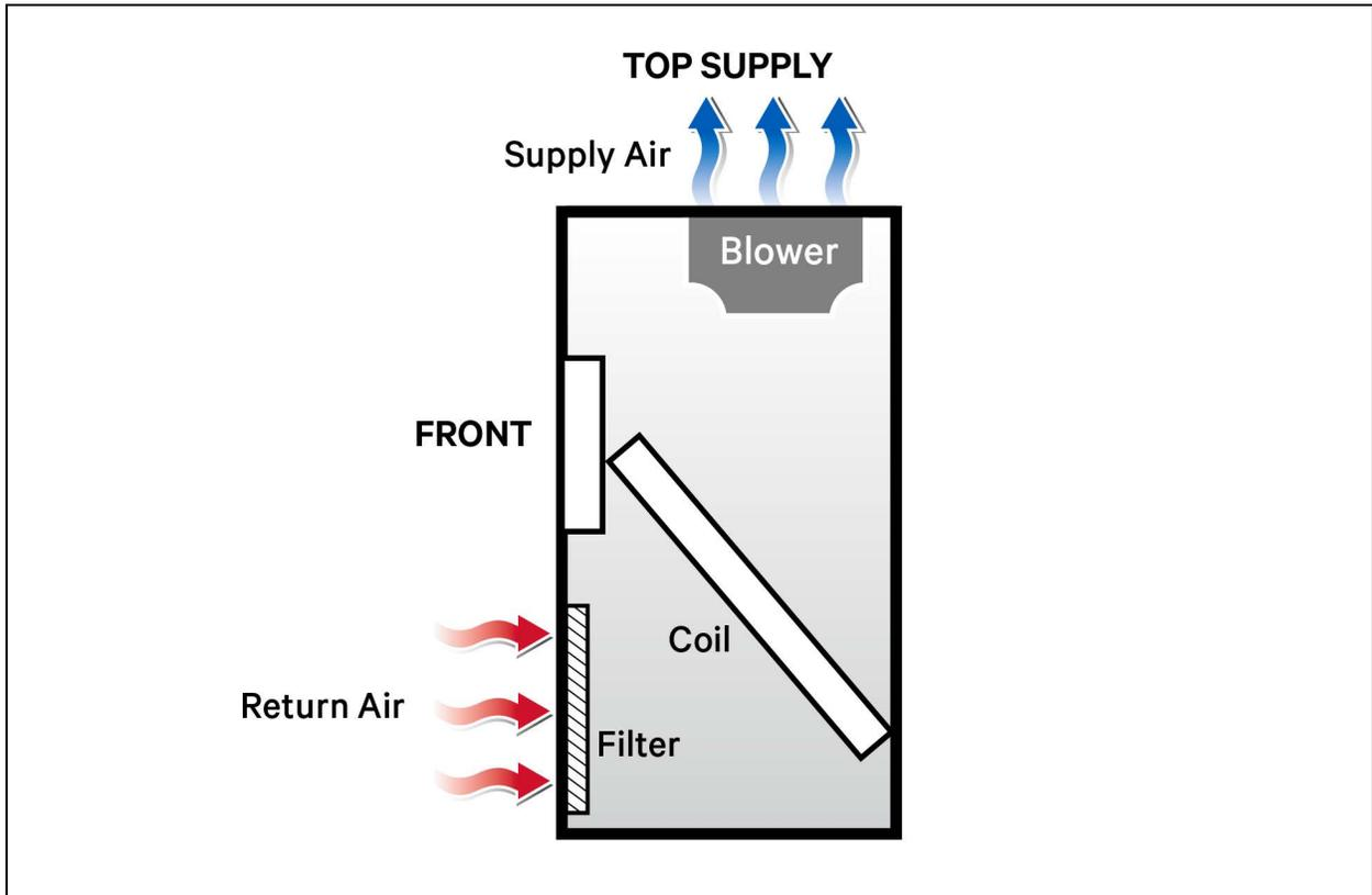
Figure 1.6 Upflow Blower Configuration, Bottom Air Return with Rear Return Floor Stand
