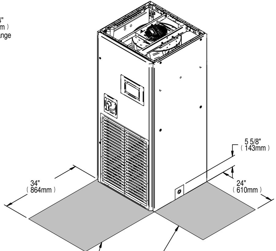
Shaded area indicates a recommended minimum clearance be provided for component access.
