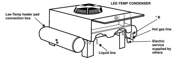
\*B - Inverted traps are to be field-supplied and installed (typ). When installing traps, provide clearance for swing end of access door. Traps are to extend above base of coil by a minimum of 7-1/2" (190 mm).
