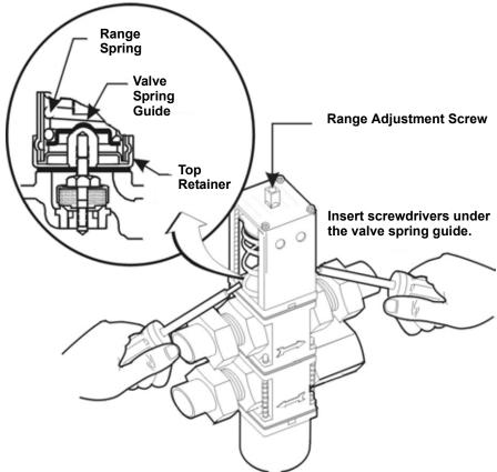
**Manual Flushing**—The valve may be flushed by inserting a screwdriver or similar tool under the two sides of the main spring and lifting. This action will open the valve seat and flush any dirt particles from the seat. If this fails, it will be necessary to disassemble the valve and clean the seat.
