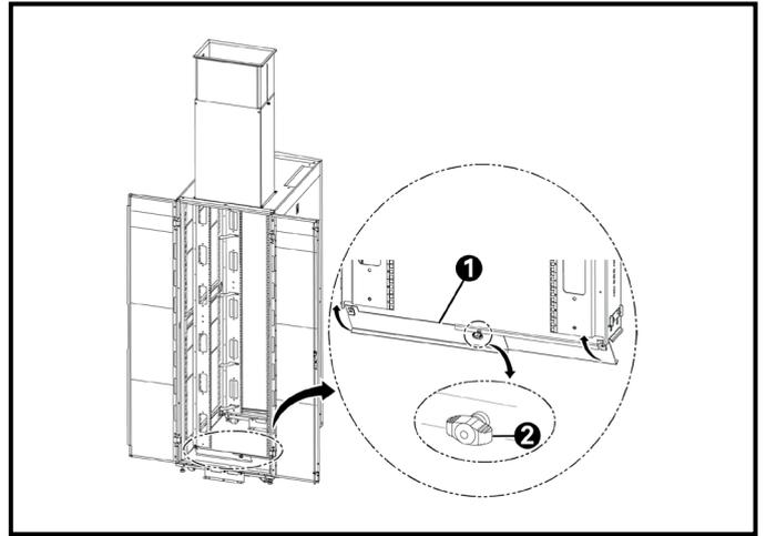
4. Install the air block panel on the bottom frame with two push-in rivets.
