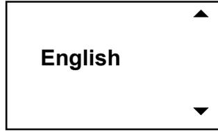
Press the “▲” or “▼” key to select the desired language. Press the **ENT** key to confirm the selection. If no key is pressed within 10 seconds, the SCU+ selects the displayed language automatically.
