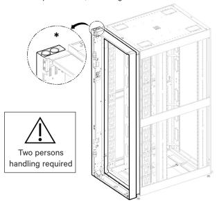
11. From DCD box, use the M5 nuts to screw both corner brackets as it shows in the image.
