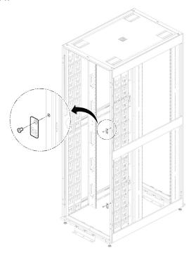
8. Discard unnecessary hardware from the DCD™ frame: all spring nuts (b), 22 M5x10 screws (a), all washers and 6 diamond nuts (c).
