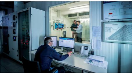
The Research & Development Validation Area n. 1 is specifically designed to test floor-mount units and can balance a thermal load of up to 150 kW with a chamber air temperature between 0°C and 60°C.
