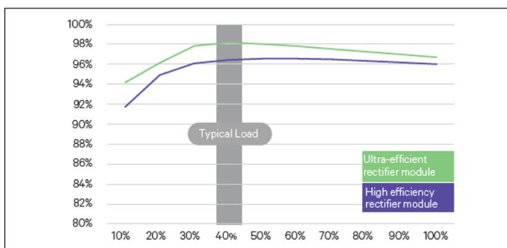
The efficiency curves of ultra-efficiency & high efficiency rectifier modules
